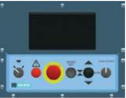
Remote connection for hoist management
